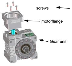
Set motorflange to the gear unit and adjust both parts via screw holes and do a precentering. Insert the screws
